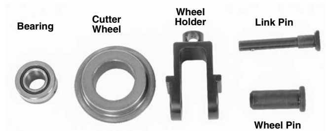
Figure 15 – Changing Cutter Wheel
