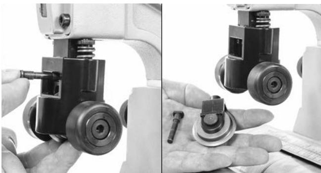
Figure 14 – Removing Wheel Holder
